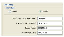
from the LAN and then connect the PC with an Ethernet straight cable using 192.168.0.101 for the IP address of the IPCMPR card.
